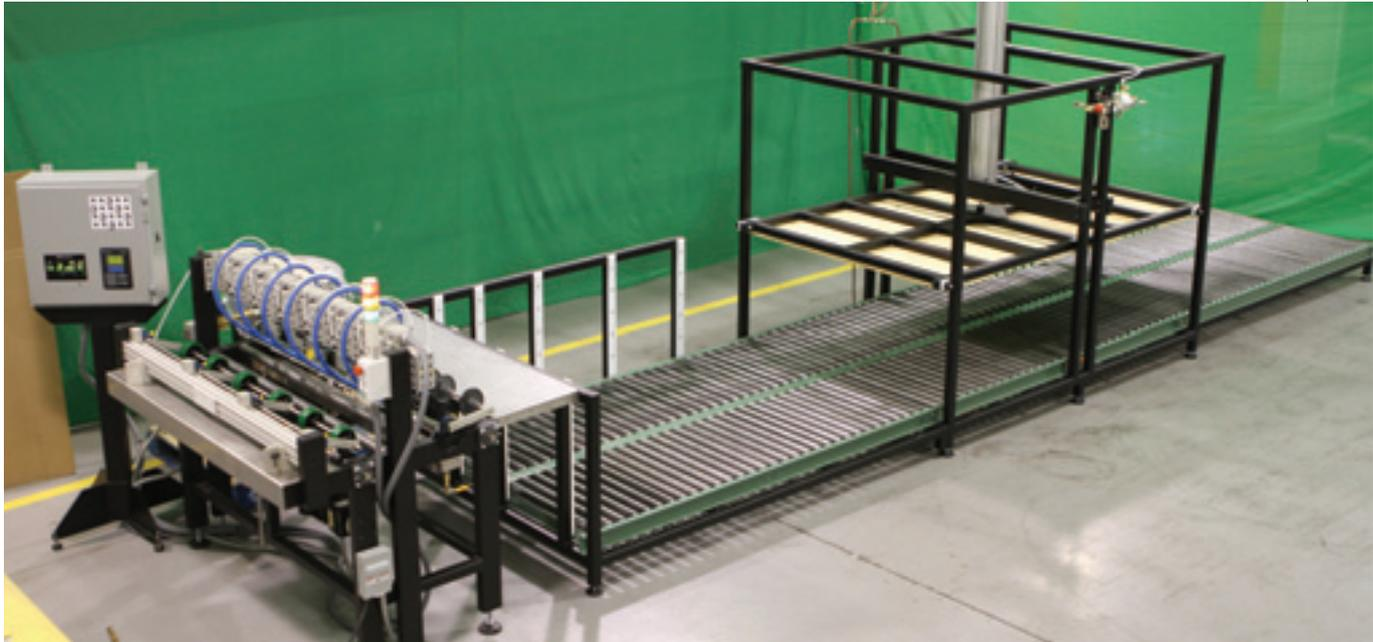
*Above: All EGS units are custom configured to customer specs in regard to sheet width, number of control channels and stacker type (either automatic or manual).*
